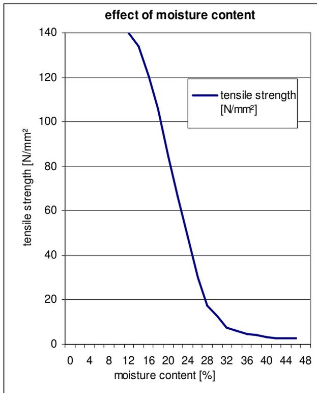
Figure 4 The effect of moisture content on the tensile strength of an animal glue that meets aircraft specification (Truax 1930)
