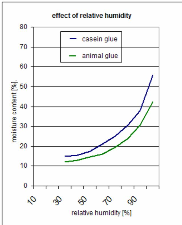
Figure 5: Effect of relative humidity on moisture content of animal and casein glues suitable for aircraft. (Truax 1930)
